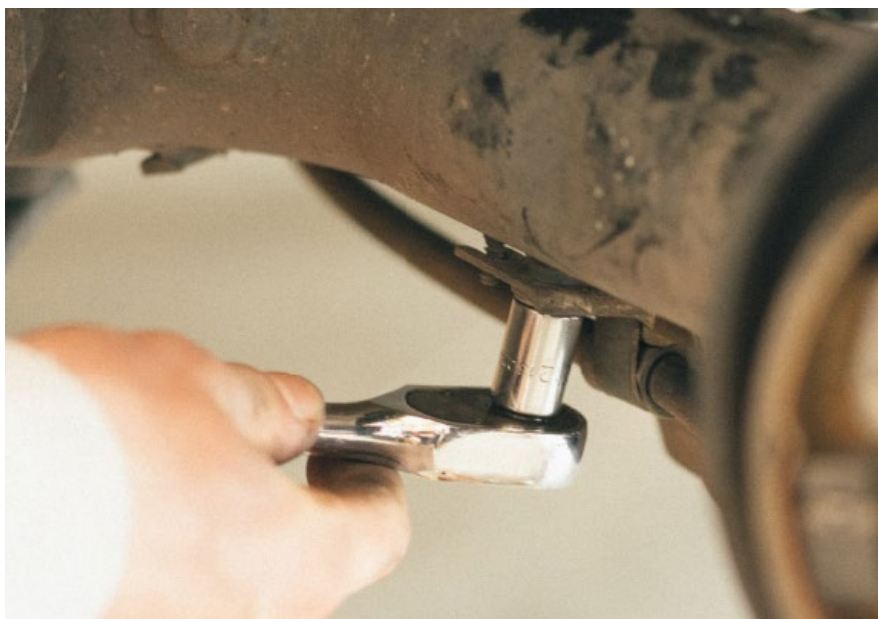
Figure 5: Rest the loose spindle as shown taking care to not damage the abs sensor or surface
