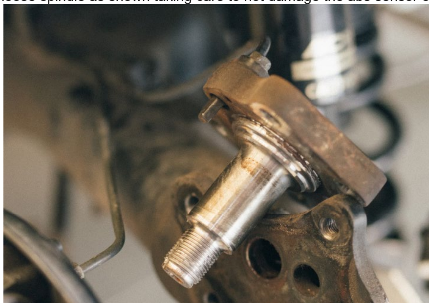
Figure 5: Rest the loose spindle as shown taking care to not damage the abs sensor or surface
