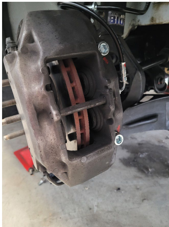
Figure 1: Front Right Caliper Orientation. Caliper Part Numbers to Bottom. Left side will have caliper part numbers on the top side
