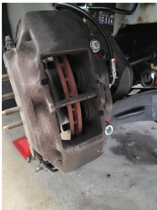
Figure 2: Front Right Caliper Orientation. Caliper Part Numbers to Bottom. Left side will have caliper part numbers on the top side
