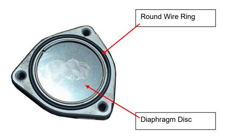
5. Remove the Diaphragm Disca. If necessary, push it out from the back with a small screwdriver.
