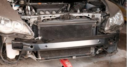
2. Using a cut off wheel, cut the crash beam as shown below:
