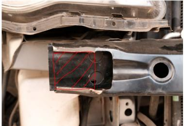
3. Mount the Tow Hook, the supplied aluminium clamp plate slides in from the side on the back face of the crash beam. The red lines below indicate the crash beam.
