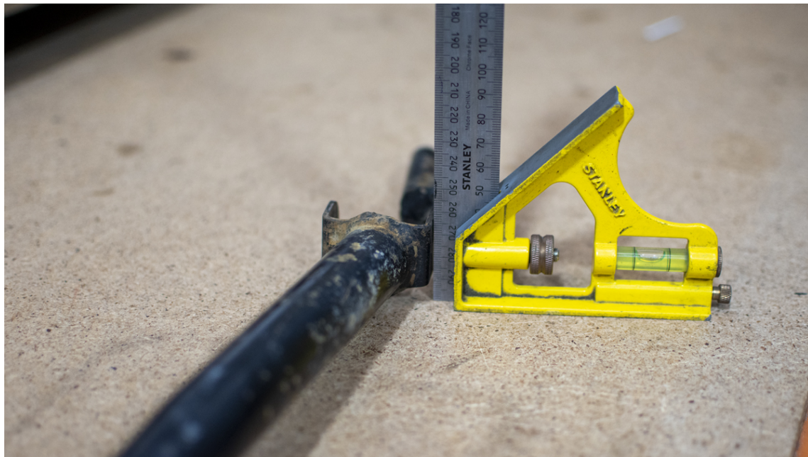
Figure 2: Square up the back of the linkage
