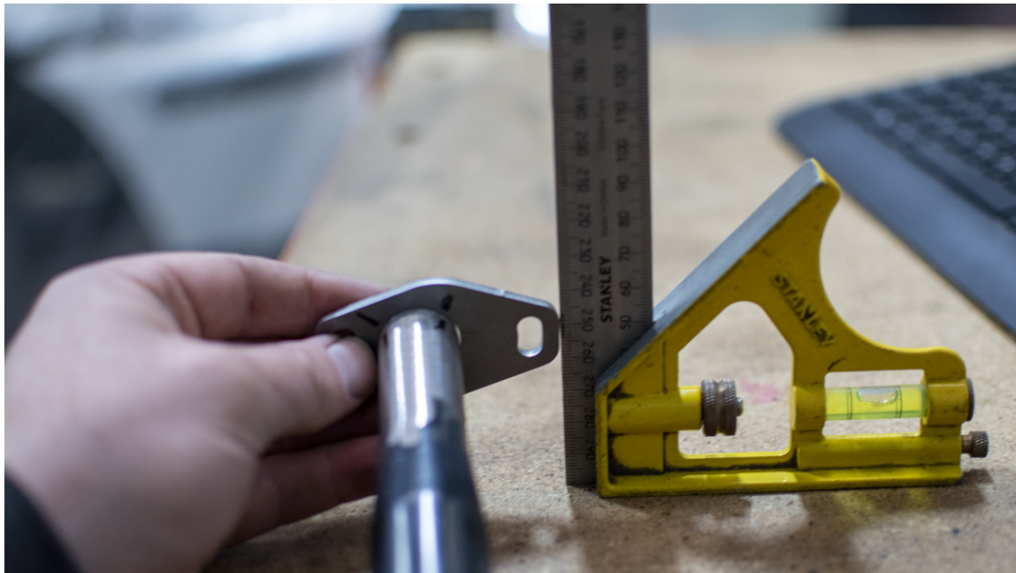
Figure 3: Align and mark the mounting plate
