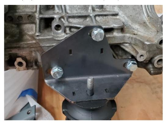
Note the location of the supplied spacers, two spacers for the top slot and three spacers for the front slot
