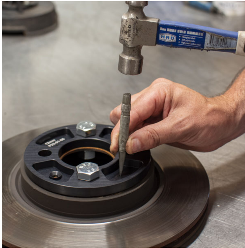
Figure 1: Using the Honed wheel spacer as a hole template
