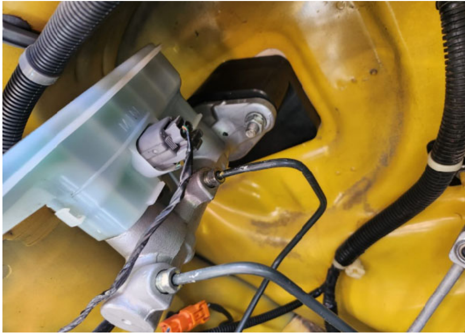
Figure 6: As installed with hardlines re-installed
