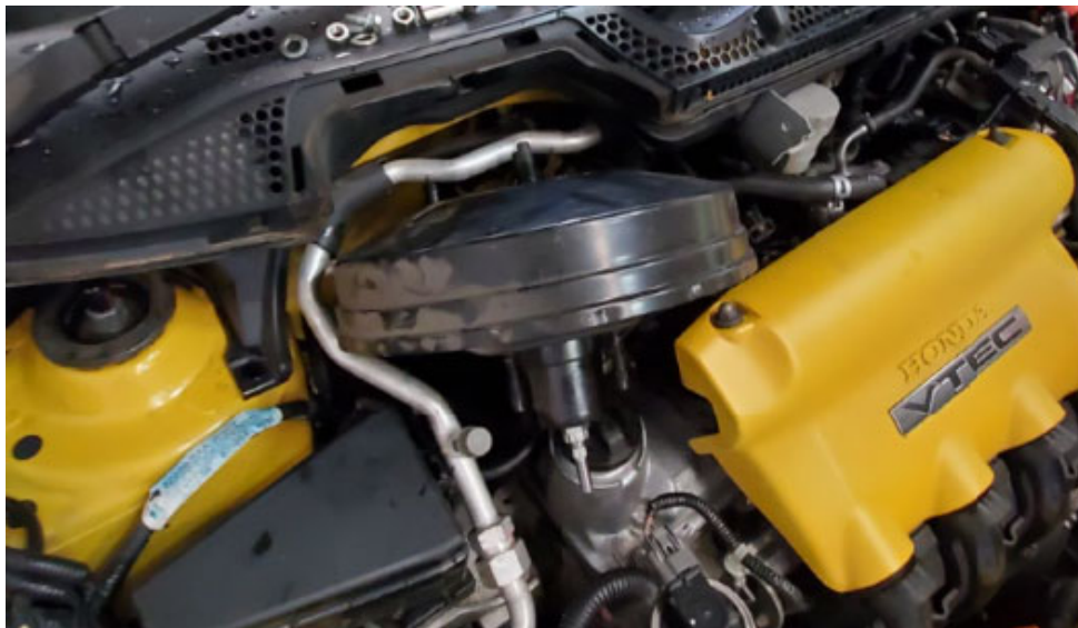
Figure 3: Orientation of booster when removing
