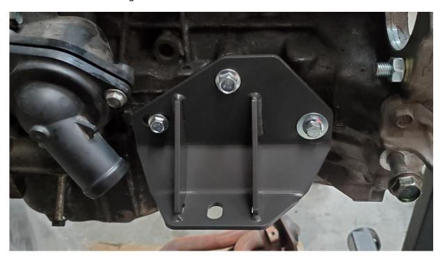
Note the location of the supplied spacers, there are four spacers used in each location shown below
