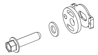
4. Tighten the bolt until eccentric housing is engaged into the body securely but washer can still be rotated
