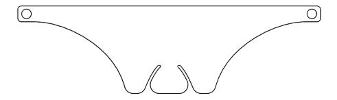
2. Bend each end of the heat shield up 90 deg as shown below
