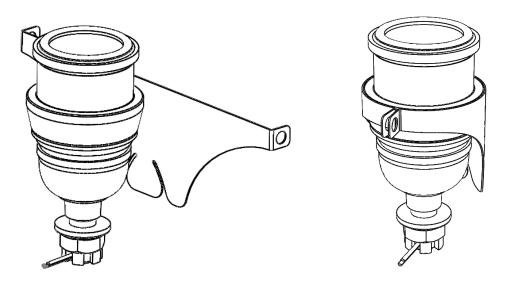
4. Install the M5 button head cap screw with washer and nyloc nut as shown.
