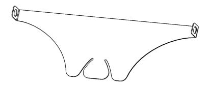
3. With the tabs facing outward, bend the heat shield around the gold collar of your ball joints
